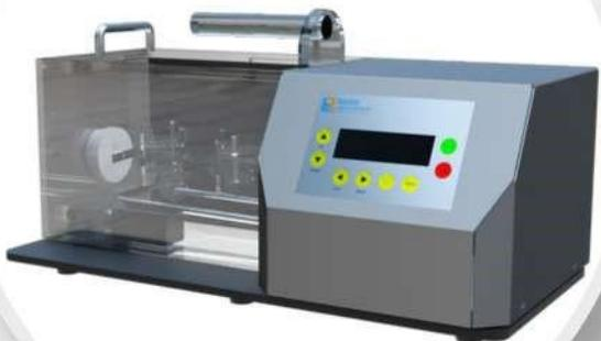
Raise Lab Equipment, the RSDT-3B is a user-friendly and compact Suppository Disintegration Tester, designed to comply with USP, BP, EP, and IP standards. Engineered with an advanced microprocessor-based design, this model ensures precise and reliable disintegration testing of pessaries and suppositories.
