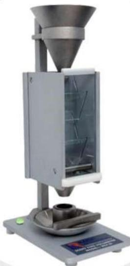
Scott Type Voltmeter is a standard bulk density tester that is extensively used in powder testing applications. The apparatus is used for determining the bulk density of free-flowing powders such as pharma, chemical powders, and compounds according to different international standards.
