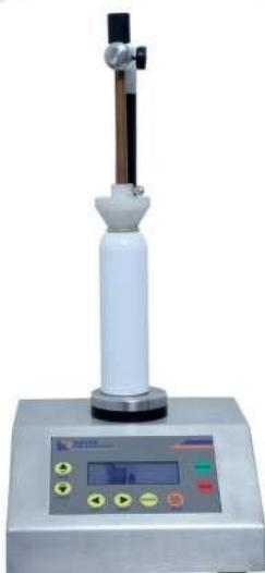
A Quality control application tool widely used to test the porosity of a Wax-coated metallic vessel in the labs. The container can be an aluminium tube, can or a bottle cap. To measure porosity of a tube means to conclude whether the wax coating has holes or spaces in it that possibly trap air or allow liquid through it.
