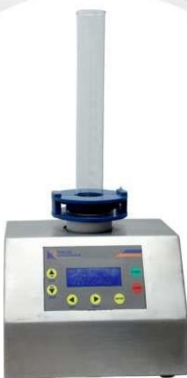
Tapped Density Apparatus measures the tapped density of materials, which is the density of a powder or granular substance after it has been subjected to a specific number of taps or vibrations under standardized conditions. This measurement provides insights into the packing characteristics of the material, including its compaction behavior and the amount of settling that can occur during handling or transportation.
