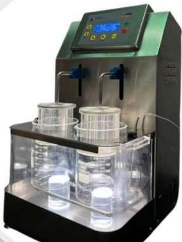
Dual Drive with 2 test baskets. Compliance with USP, EP, and other pharmacopoeia. Compact design with splash-proof keypad. 20x4 LCD screen with backlight. Quick release basket and auto-parking. Online validation of strokes per minute. Safety features, bath illumination. External probe for temperature validation. Printer port, RS 232 interface for reports. Password protection for Real-Time Clock. IQ/OQ documents.
