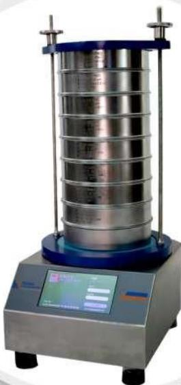
Electromagnetic sieve shakers use electromagnetic forces to generate vibrations, facilitating particle size analysis by separating materials based on size as they move through a stack of sieves with varying mesh sizes.
