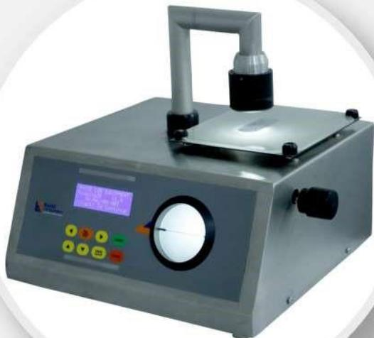
The antibiotic zone reader provides an immediate and accurate method for determining the strength of antibiotic materials by measuring the diameter of an inhibition zone in a Petri-dish.
