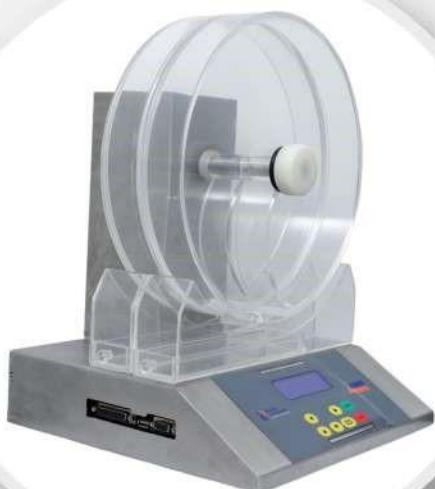
Tablet friability testing is a crucial parameter in quality control in the pharmaceutical Industry. It involves subjecting tablets to mechanical stress in order to assess their durability and resistance to breakage. This testing ensures that tablets maintain their integrity during handling, packaging and transportation. Furthermore, tablet friability testing is required by Pharmacopeia standards such as British Pharmacopoeia (BP), United States Pharmacopoeia (USP) and Indian Pharmacopoeia (IP).
